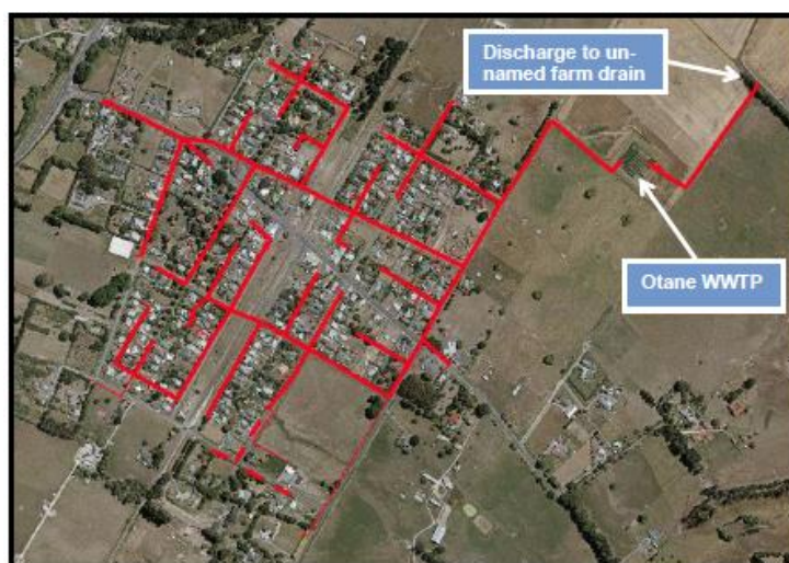
Layout of the Otane wastewater network
