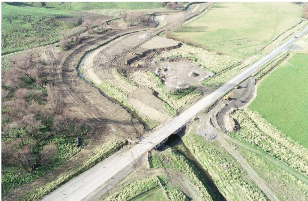
Figure 4: Flaxmill Bridge clearing and silt removal
