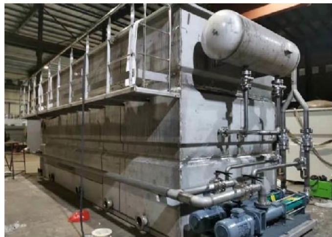
Figure 1: Waipawa DAF unit being fabricated in China
